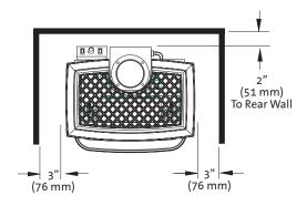
Figure 2. Parallel Installation Clearances.
